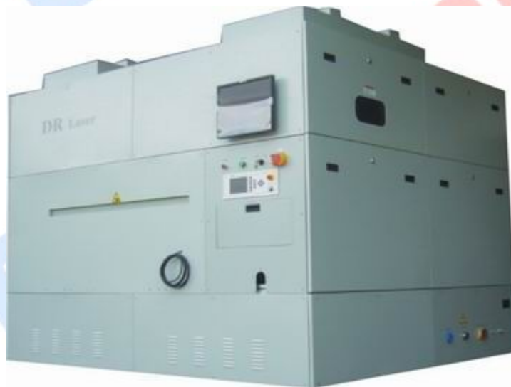
Application: Laser scribing for Thin film solar cells P1 /P2/ P3.
